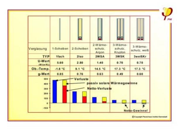
Another key technology in good houses is excellent window insulation. Windows consist of three layers, so there are two spaces between them. The hollows are specially treated on one side so that heat is not transmitted to the other side by means of radiation. Heat conduction within each space is suppressed by filling the space with a less conductive gas, ideally krypton.
